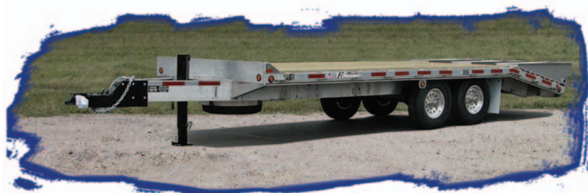
▲ FT-14A TAG 8' x 16' + 5' beavertail with optional center ramp, spare tire mount, aluminum rims, stake and strap.
