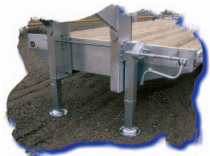
Twin 140,000# 2-Speed Landing Gear Standard on FT-18 and Up
