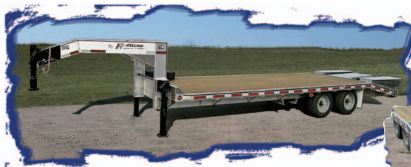
▲ FT-16A GN 8'6" x 24' + 6' beavertail with optional center lift and slide out center ramp.
