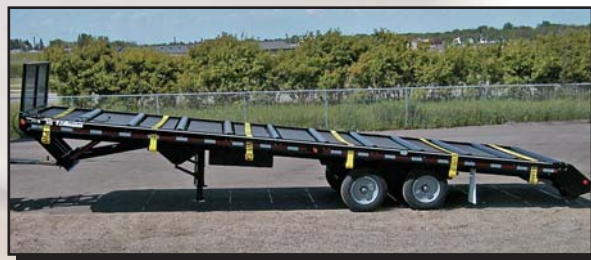
FT-16 IT with stationary platform optional spare wheel & tire, gooseneck, Omaha Orange paint and twin 12,000 lb. drop-leg jack.
