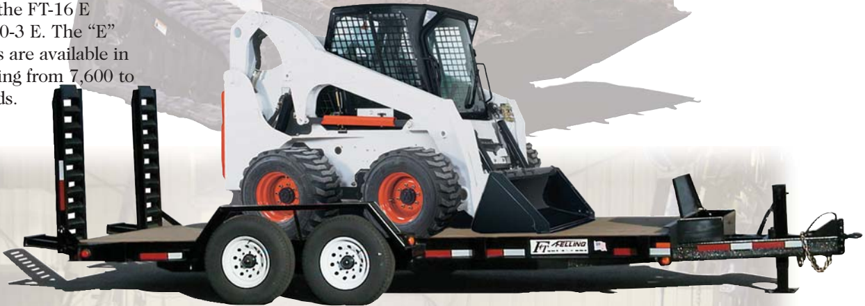
FT-12 E with optional 84” wide deck, HD channel fenders with open wheel wells, lockable toolbox and standard 12,000# jack.
