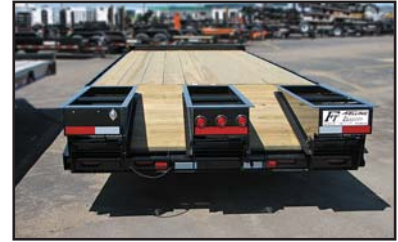
FT-12-2 with standard wood inlaid beavertail and ramps, and optional center ramp.
