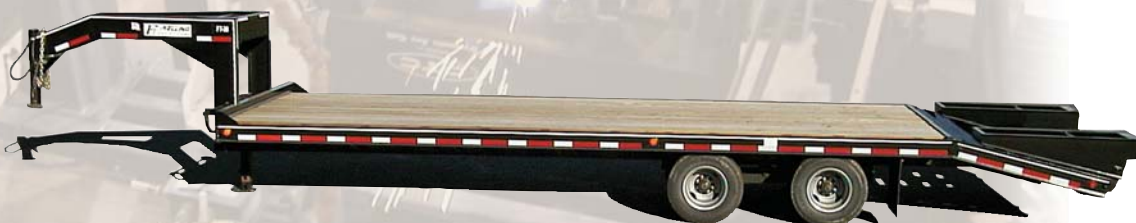
FT-20-2 GN Farm & Ranch with 5' beavertail, 5' spring-assist ramps, standard stake pockets inside channel (shown on the left) and optional 12,000 lb. jack.
