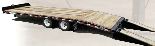
FT-40-2 LP shown to the left and below with optional a double inclined, wood inlayed beavertail and wood inlayed ramps. This trailer also has a lower loaded deck height of 33" vs. the 35" height of a standard FT-40-2.
