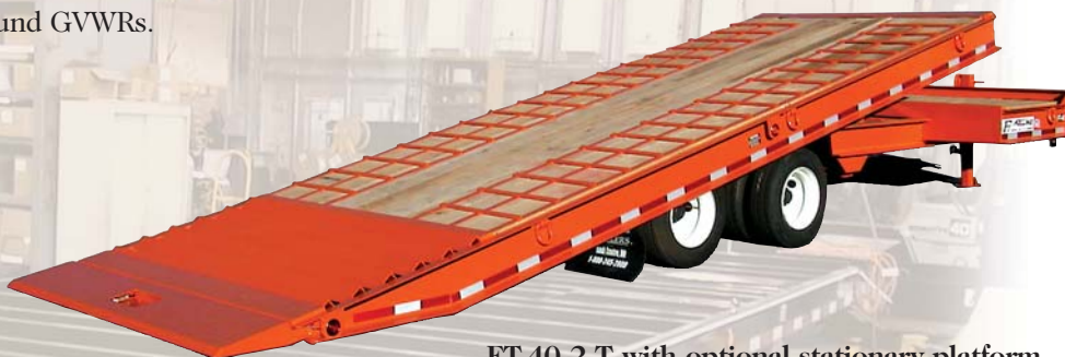
FT-40-2 T with optional stationary platform, 5" x 3" self cleaning angle on tail section and white oak on remaining deck and traction aids.
