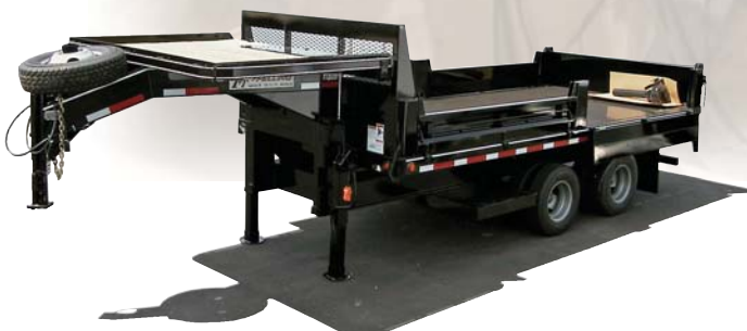
Above: FT-20-2 DT-C GN with Contractor Body OPT Upper Deck & Spare Wheel/Tire
