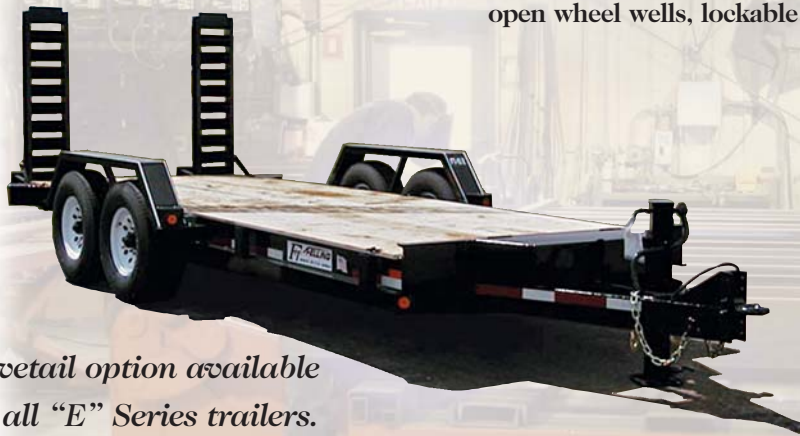
FT-12 E with optional 84” wide deck, HD channel fenders with open wheel wells, lockable toolbox and standard 12,000# jack.
