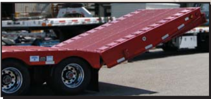
FT-80-2 PL HT (Perimeter Frame-Hydraulic Tail) with opt. double drop deck, upper hydraulic deck and winch.
