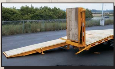
FT-50-3 with OPT 11' hydraulic bi-fold wood inlayed ramps, wood inlayed beavertail and front air lift axle.
