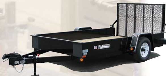
FT-5: 80" x 12' with Std. electric brakes
