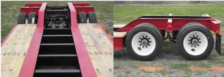
■ Lowered crossmembers in the rear frame provide extra space for excavator booms. "Lumber to the tires" yields an extra foot of deck space. Light-weight trunnion beams are used to tie-down loads. Spring loaded parking brakes provide improved loading and unloading safety.
