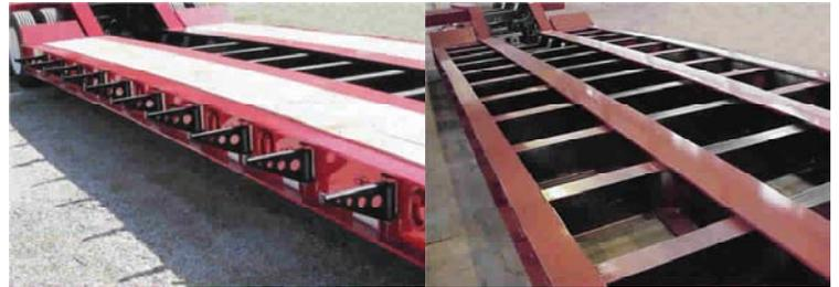
■ Unitized frame with mainbeams fabricated of 100,000 PSI steel. Heavy-duty, full-width cross members on 24" centers for longer deck life. Full 1 3/4" air-dried oak decking installed with carriage bolts and cupped washers for easy replacement. Optional heavy-duty swinging, removable cast side brackets widen the deck to 10'- 6". Tested and certified D-rings exceed today's load securement regulations.
