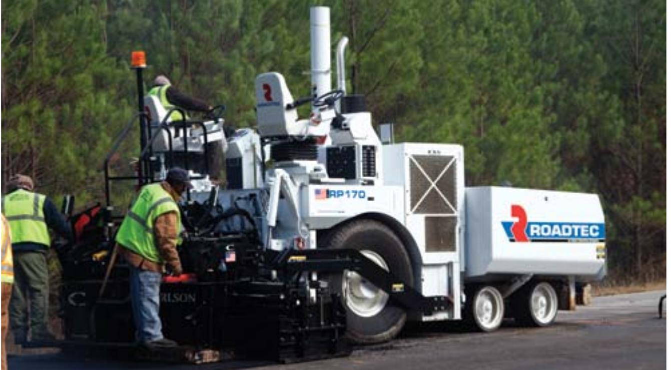
The RP-170 is a rubber-tire asphalt paver with a compact wheelbase for great maneuverability. The RP-170 can achieve a 30" (76cm) turning radius for managing those tight spots around barriers and drains. Fume extraction, adjustable seats, and quiet operation. Quick and easy transportation between job locations.
