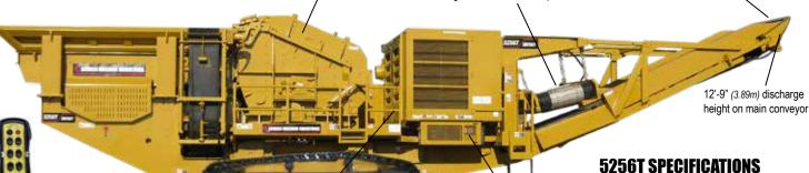
Heavy-duty tracked undercarriage with easy-to-use wireless remote control, for quick and efficient set-up and operation
