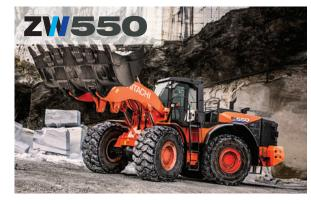
Bucket Capacity .....8.3-9.0 yd<sup>3</sup> Operating Weight. . . . 104,570 lbs Engine Output, Max, Gross 520 HP Breakout Force . . . . . . . 83,460 lbs
