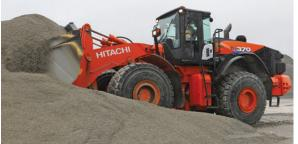
Bucket Capacity ..... 7.3–8.1 yd<sup>3</sup> Operating Weight. . . . . 73,789 lbs Engine Output, Max, Gross 389 HP Breakout Force ......51,931 lbs
