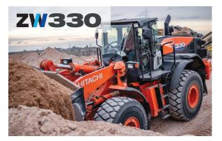
Bucket Capacity ..... 6.3–6.8 yd<sup>3</sup> Operating Weight. . . . . . 58,158 lbs Engine Output, Max, Gross 311 HP
