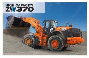
Operating Weight. . . . . . 79,010 lbs Bucket Capacity .....8.1-8.5 yd<sup>3</sup> Engine Output, Max, Gross 389 HP Breakout Force . . . . . . 49,280 lbs
