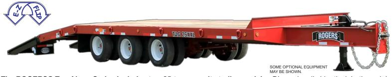
The ROGERS® Tag-Along Series includes two 25-ton capacity trailer models. Dimensionally identical, both models exhibit superior construction with the use of high strength steel beams and integrated frame design. The TAG25XXL utilizes a heavy-duty spring suspension on all three axles while the TAG25XXL-AL incorporates an air suspension with air lift on the front axle. Better load distribution and extra-long loading ramps mean safer and easier operation.
