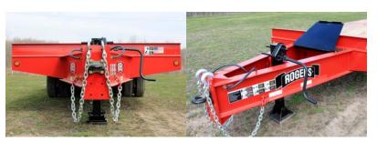
Longer drawbar & premium landing gear: Longest drawbar in the industry makes for better load distribution and easy handling. 1/2" safety chains are integral to the frame of the trailer, not welded or bolted in place. The two-speed landing gear has 50,000 lb. lift capacity and 70,000 lb. static capacity. The pintle eye adjusts to accomodate various heights using standard shop tools. There is ample room for chain and tool storage in the drawbar toolbox with lockable steel lid.
