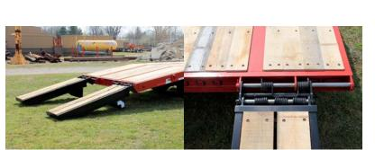
Extra-long loading ramps with 72" beavertail at 8° slope: Constructed from high-strength 50,000 psi minimum yield steel, these ramps are strong and durable yet lightweight for easy operation. Dual springs assist the operator lifting the ramps off the ground as well as off the deck. The ramps can be easily adjusted laterally to handle machines of various widths. Extra length reduces the climb angle for safer loading. These "E-Z Flip" ramps are standard oak-covered or optional ladder style.
